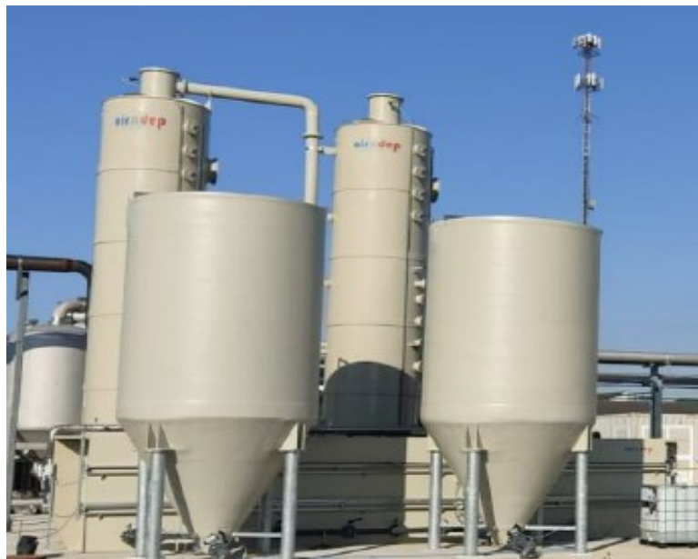
Figure 14: A two-stage H 2 S scrubbing system
