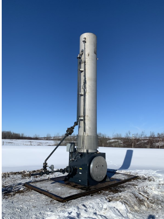
Figure 17: Example of a safety flare
