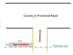
The address sign should be 60 x 30 cm in dimensions with minimum 080 aluminum that is engineered-grade reflective surface. It should have a white reflective letter on a medium blue background, pre-drilled 3/8-inch holes on 2 or 4 sides for installation with a 1.5-inch corners; and no borders.
