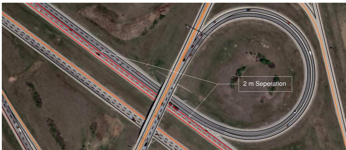
Figure 10.1: Ramp Merge Physical Separation Concept
