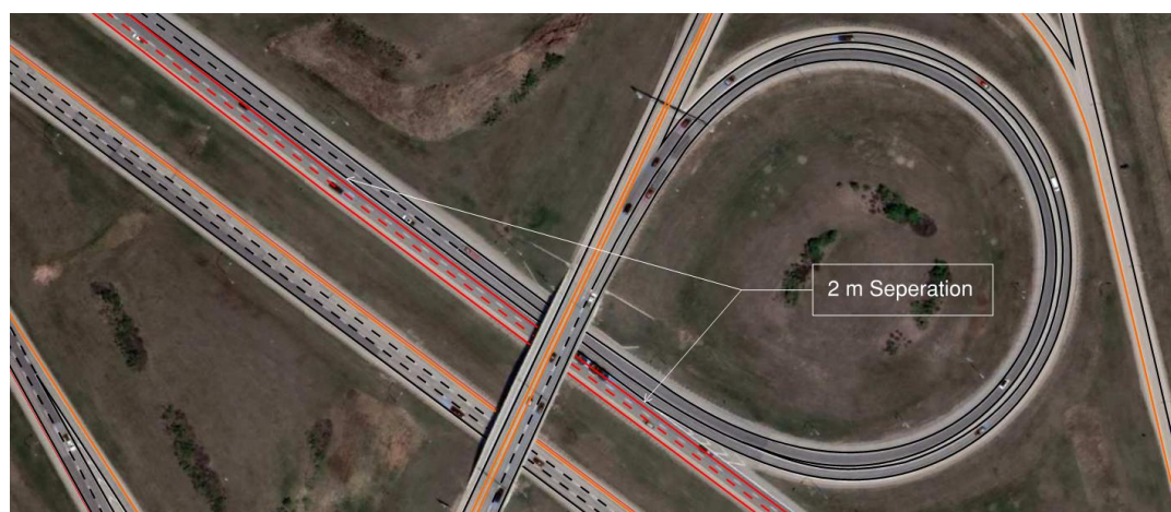
Figure E4.1: Ramp Merge Physical Separation Concept
