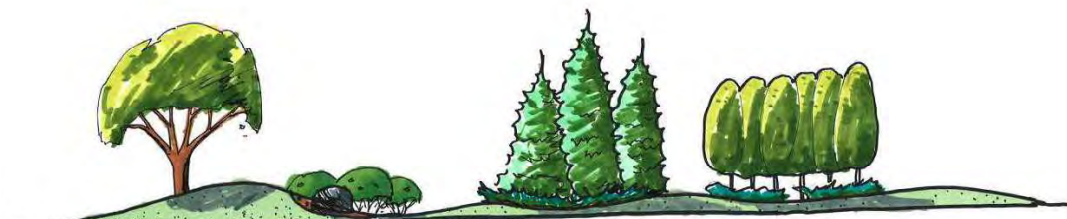
0 5 10 m Combination Screen – Full, Partial or Buffer Screening (Earth Berms and Mixed Planted Landscaping)
