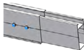
Then use two sets of Self-tapping screws in each side of the T Rail
