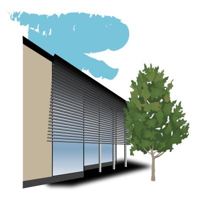
Fig.18 An example of an exterior design that reduces solar heat gain.
